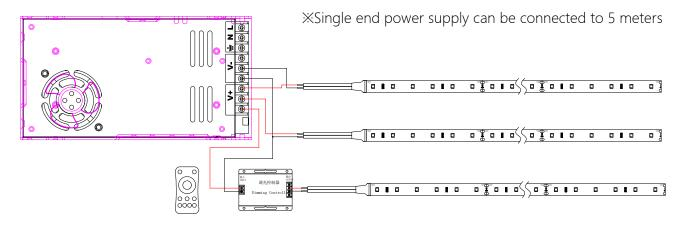
\*The dimmer can be connected to achieve dimming
